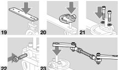
→ Do not fully tighten the lever for the butterfly valve.
